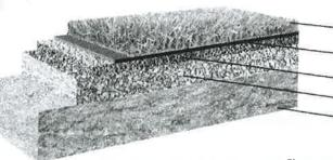
Artificial Grass w. Sand Infill Membrane Granite Gmm - Dust Type I Stone Compacted Soil
